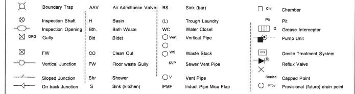
NOTE Further acceptable abbreviations may be used as identified in AS/NZS 3500.2.2003 Sanitary Plumbing and Drainage
