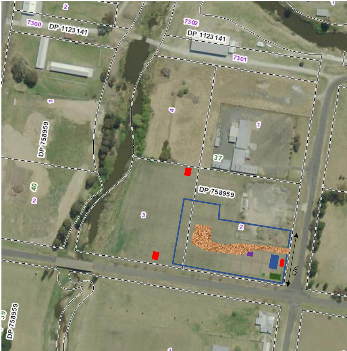
Figure 4: Site layout showing custodian site, shelter, storage shed, dump point and internal driveway
